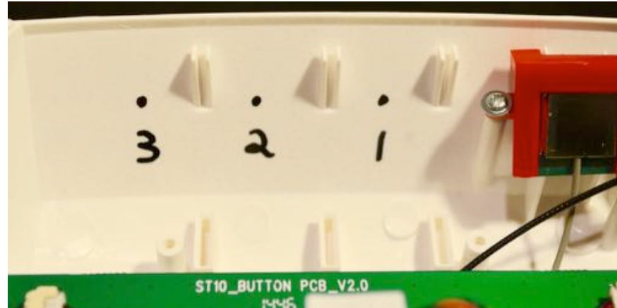
Step 13: USE Marker to mark drill holes for connectors. Good reference to number them for Port Assignment
