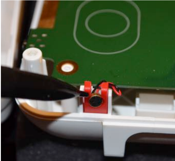
Step 11: CAREFULLY slot the MIC back into position
