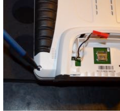
Step 3: Remove 6 screws Larger ones from unit
