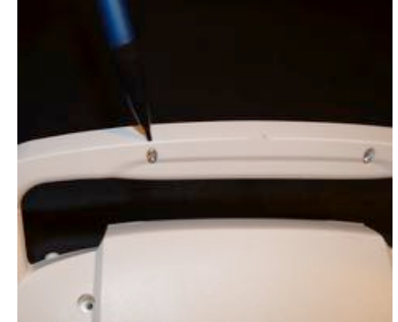
Step 4: Remove 2 screws Small ones from top handle
